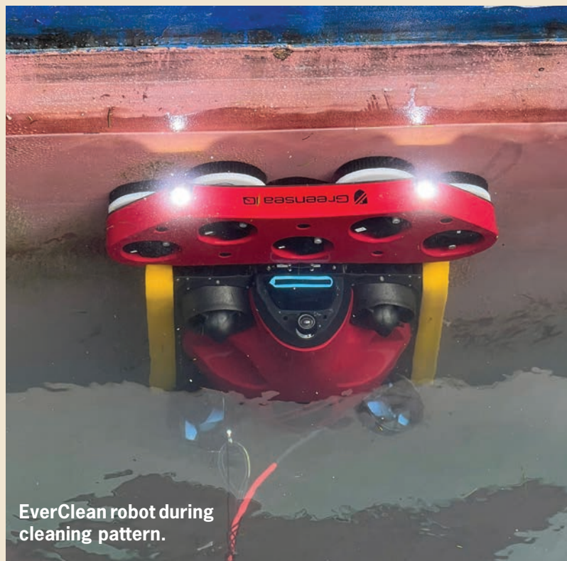
EverClean robot performing cleaning on ship hull in Port Canaveral, Florida.
