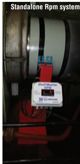
Standalone Rmp System that has (4-20 ma output) to the bridge and or control room to our touchscreen. Total, revolutions, direction and instantaneous Rpm for Maneuvering, Shaft Stop (optional) specific fuel consumption. Local and remote touchscreen bridge and control room viewed by 3.5” or 7 in” typical.
