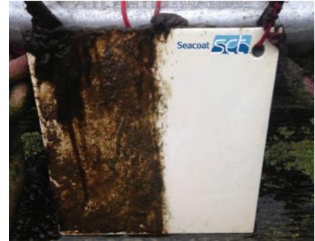
(L to R): Photos of static testing of the SEA-SPEED V 10 X ULTRA based on two diametrically different fouling environments. The first is a 90-day static panel cleaned with a sponge, mid-Atlantic coast of France. The second and third are 6-month static immersion in Coral Sea waters of Cairns (NW Queensland) Australia. You have a pre-wipe and finger post-wipe photo. This one is particularly interesting as there is virtually nothing on it in a very aggressive fouling environment.
