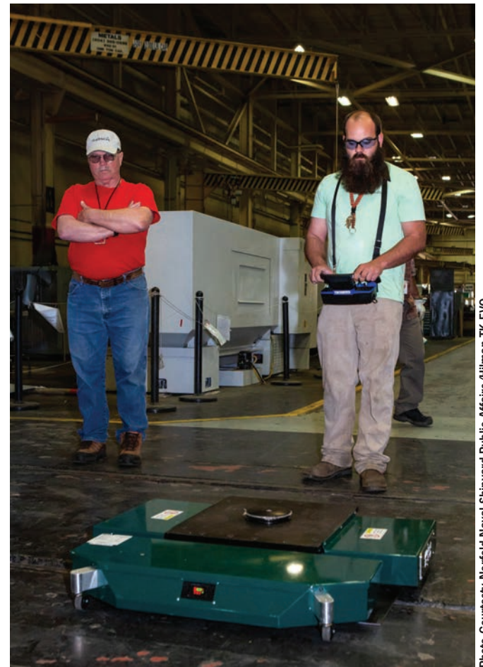
Production Machinery Mechanic Ethan Holland operates the TK-EVO Heavy Lifting Device using a remote-controlled device.
