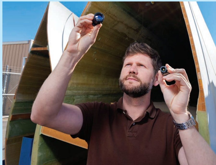
Ray Ely of Sandia National Laboratories inspects the cameras to be tested on drones that use thermography to detect hidden wind blade damage.
