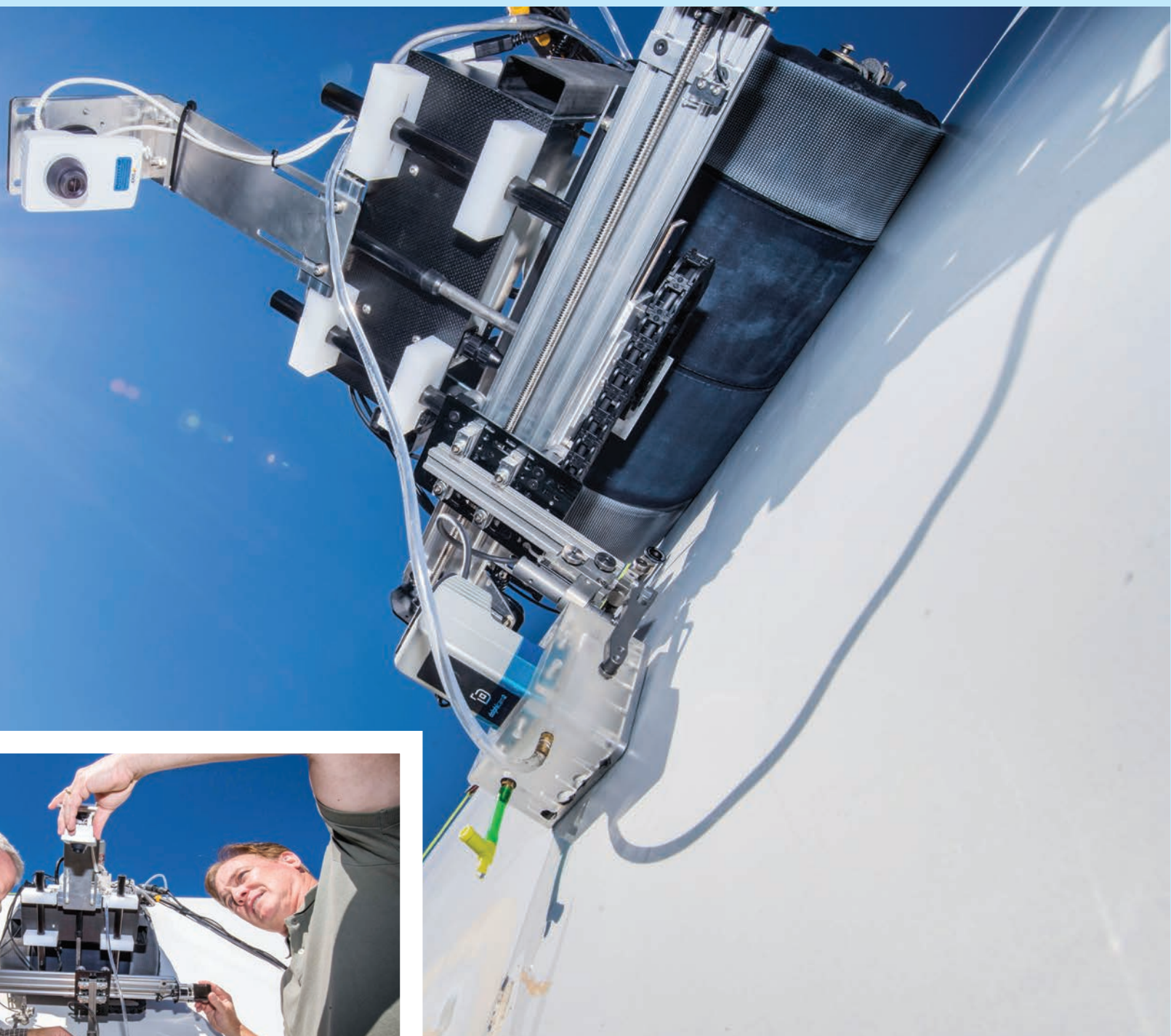
Sandia National Laboratories researchers use crawling robots and drones with infrared cameras to look for hidden wind blade damage to keep blades operational for longer and drive down the costs of wind energy. INSET: Tom Rice, left, and Dennis Roach of Sandia National Laboratories set up a crawling robot for a test inspection of a wind blade segment.
