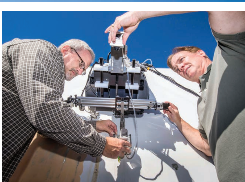
Sandia National Laboratories researchers use crawling robots and drones with infrared cameras to look for hidden wind blade damage to keep blades operational for longer and drive down the costs of wind energy. INSET: Tom Rice, left, and Dennis Roach of Sandia National Laboratories set up a crawling robot for a test inspection of a wind blade segment.
