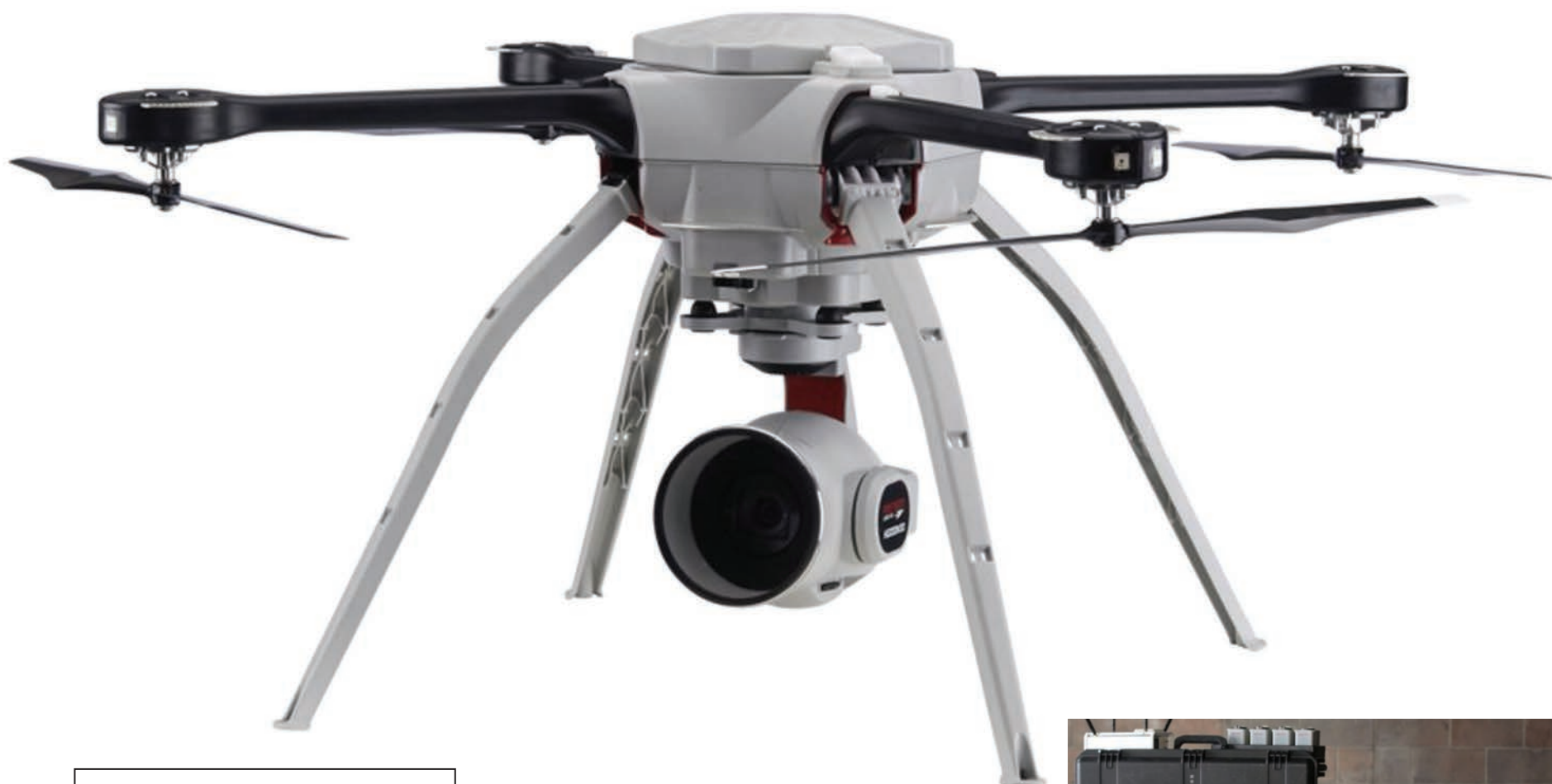
Complete sulfur-sniffer package: A NAS emissions inspection drone made from a modified Aeryon Labs R70 drone; below the original R70. Image: NAS/The Norwegian Coastal Administration Image: NAS/The Norwegian Coastal Admin
