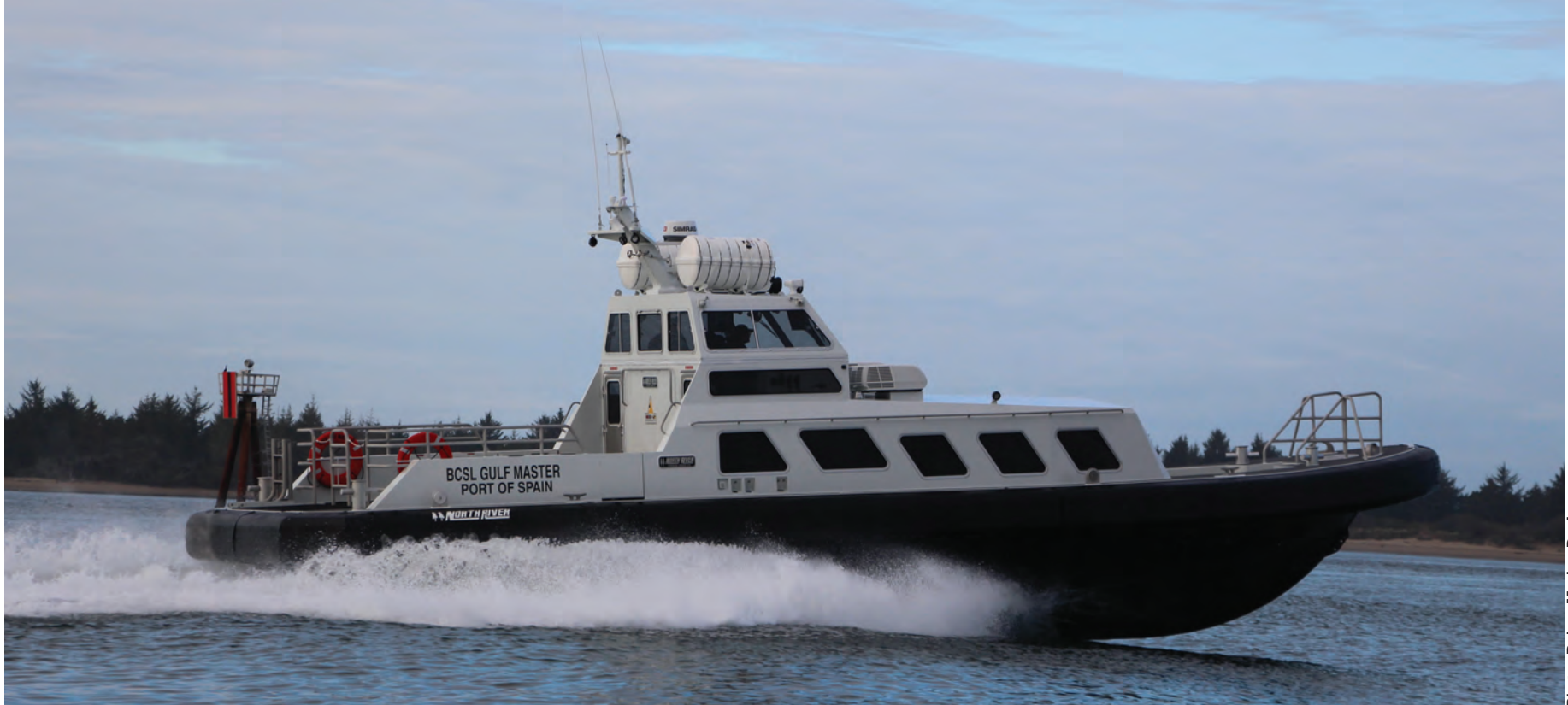
BCSL Gulf Master 58 by North River Boats, for pilots association transporting crew in hostile waters near Venezuela. Naval architecture and marine engineering by Boksa Marine Design.
