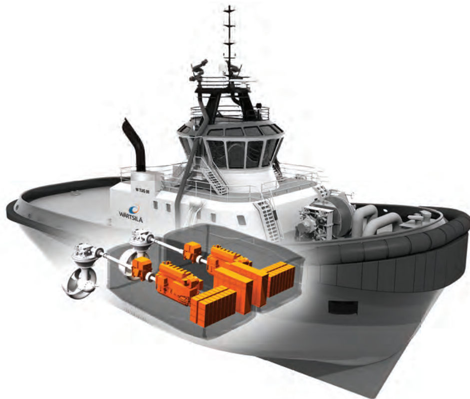
A typical system arrangement with the Wärtsilä HY for a tugboat application, in diesel-mechanical configuration with shaft motor/generator.
