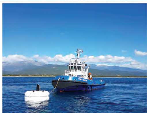
A tug is connected to the buoy for pre-tensioning.
