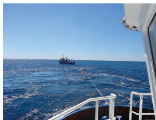
The RLP was used to measure pre-tension up to 30t to check anchors were set properly.
