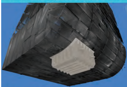
Cofferdam model fitted to FPSO hull scan. Perfect fit is verified before repair begins.
