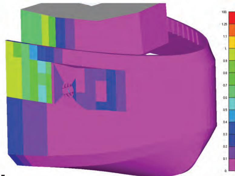
Figure 5: Color Coded Buckling Assessment Plot using ABS Rules for Multiple Load cases.
