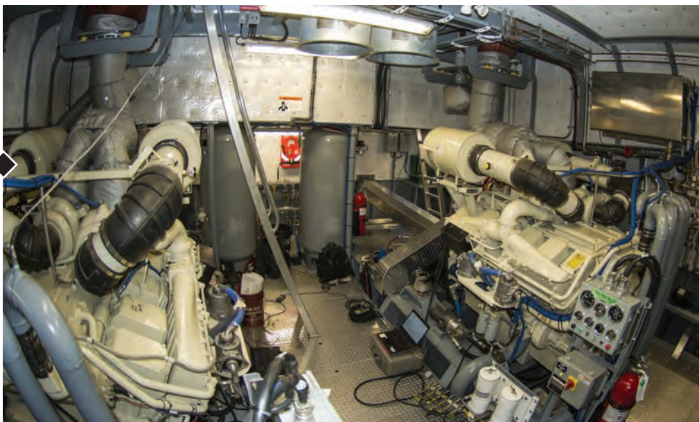
The David J's twin 1200 HP Cummins KTA38 mains.
