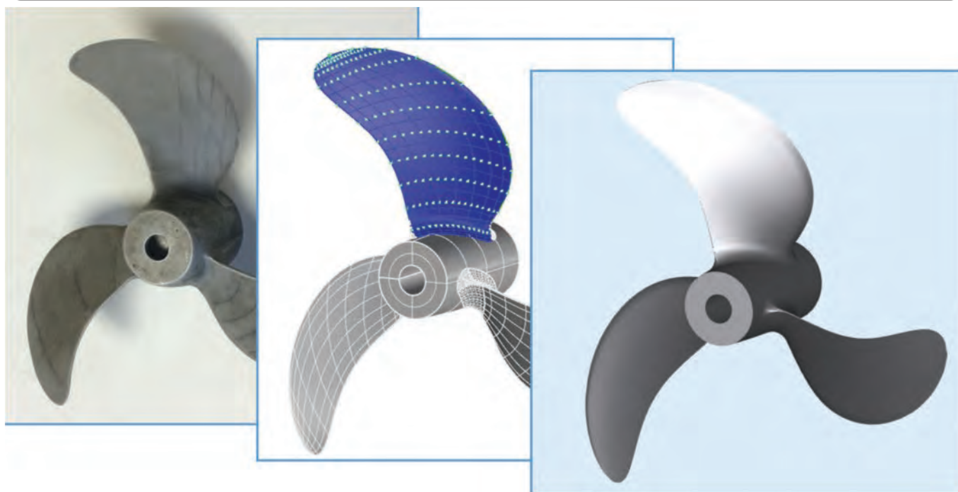
Figure 2: Scan Converter can be used to extract the design parameters and recreate the blade.
