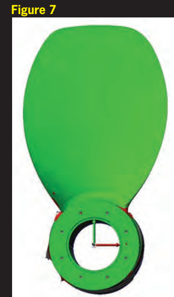
Figure 5: 3D scan of existing blade.
