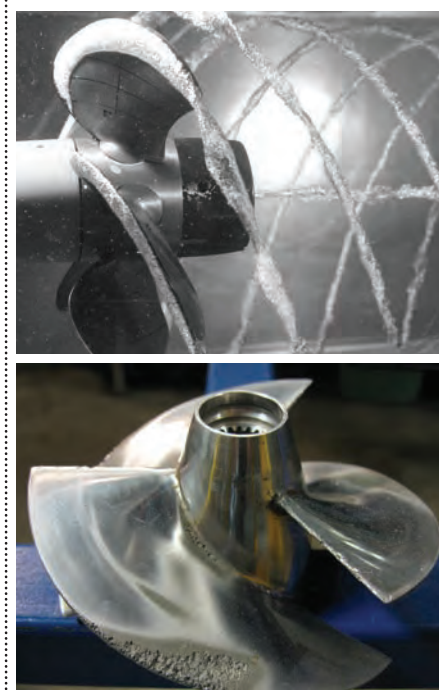
Figure 4: Tip vortex and blade back cavitation (left), and cavitation damage (right)
