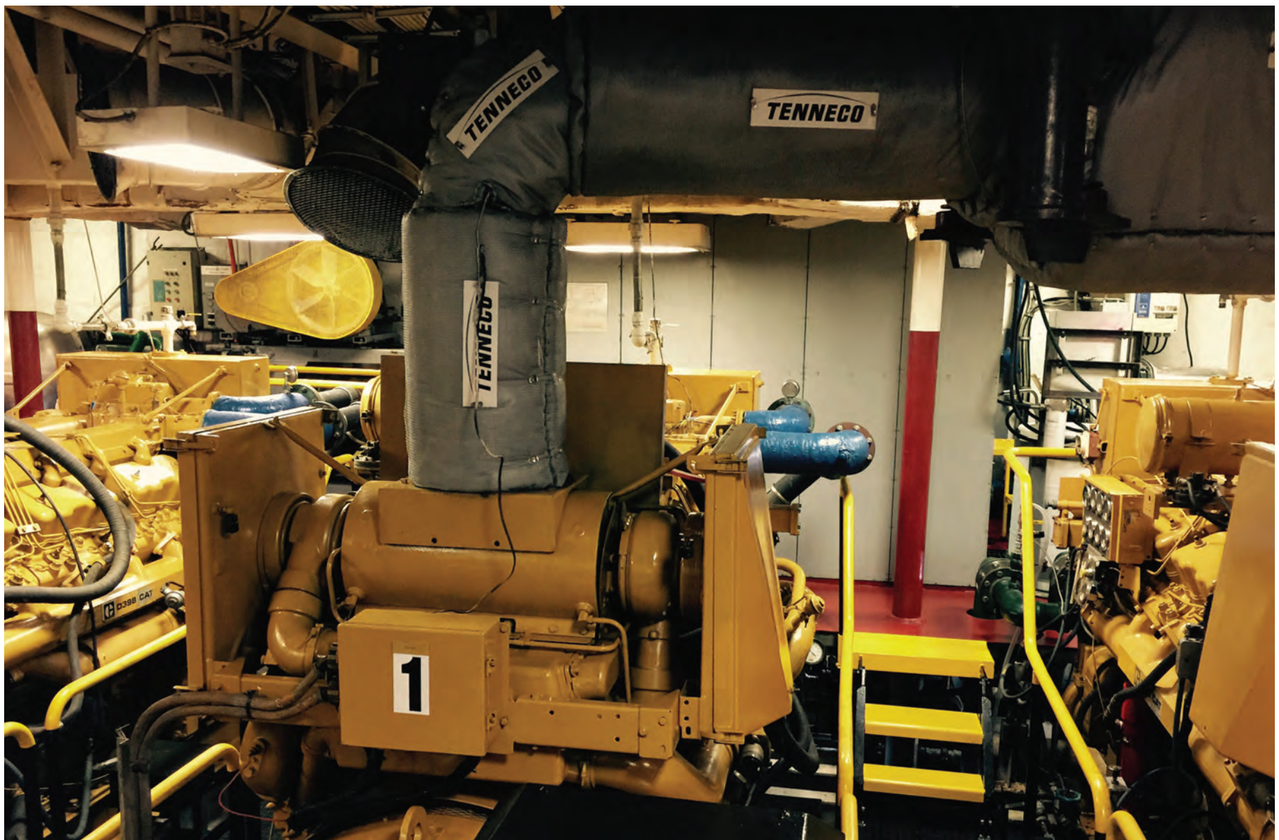
TS General Rudder is powered by four, 1982 Caterpillar 800 hp, tier 0 diesel engines.
