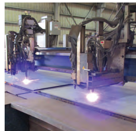
Eastern Shipbuilding and Great Lakes Dredge & Dock Company cut steel starting the construction of a new 433-ft. Trailing Suction Hopper Dredge ATB. To be named Ellis Island (ESG Hull 253), the detailed engineering is being performed by Bay Engineering, Inc., and is based upon an Ocean Tug & Barge Engineering, Inc. ATB design. Delivery is expected in 2016.
