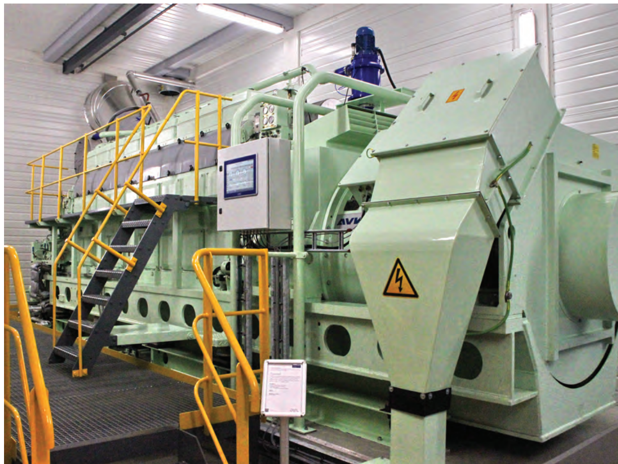
Left: View on the inline PureSOx scrubber arranged in the test facility. Right: The heart of the center: a MAN 9L28/32 engine which is coupled to a AvK-Generator with an output of 1,880 kW at 750 rpm.
