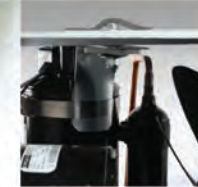
Compressor stabilization for protection in heavy seas
