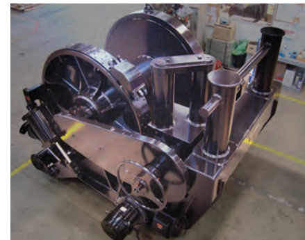
As the new year begins, Markey Machinery is preparing a new TES-40-75HP electric towing winch for shipment that will be installed on Harley Marine Services new Z-drive ship assist tractor tug "M/V ROBERT FRANCO."
