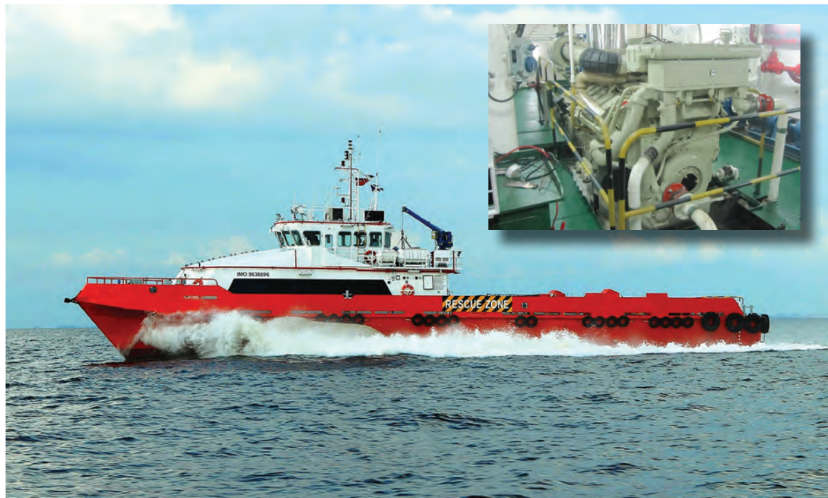
A new Cummins-powered aluminum crew boat from Sarawak Slipways. Inset: The port-side Cummins KTA38-M2. One of three main engines on Sarawak Slipways new 4500 HP crew boat.
