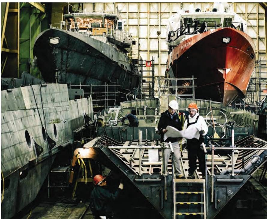
Inside the Module Shop where Canadian Coast Guard Hero Class Mid-Shore Patrol Vessels are currently being constructed.
