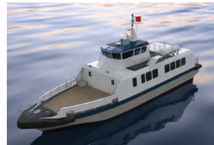
The 25m Fast Crew Boats are powered by MAN engines driving 4 Rolls-Royce waterjets.
