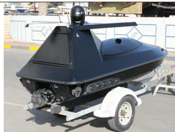
ABOVE The 3m, 60+ knots Sea Serpent USV.
