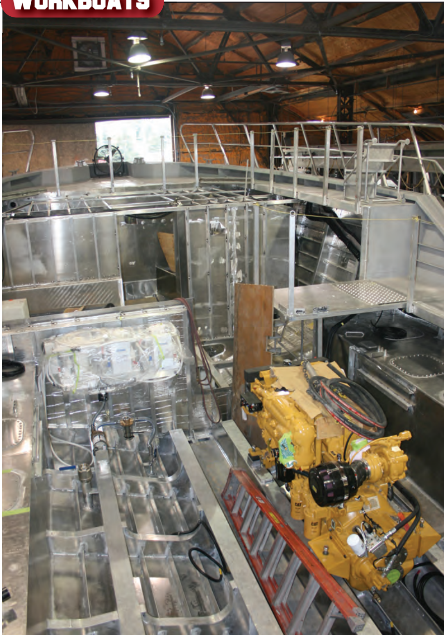
A 70-ft. Fireboat under construction at MCM's Kingston, Ontario facility.
