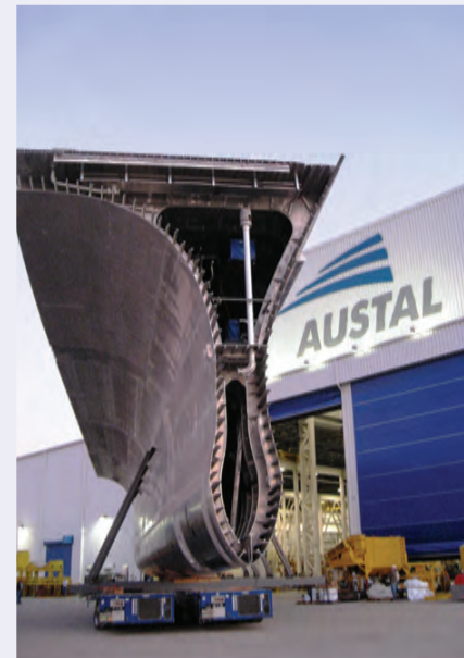
Above JHSV module on the move.
