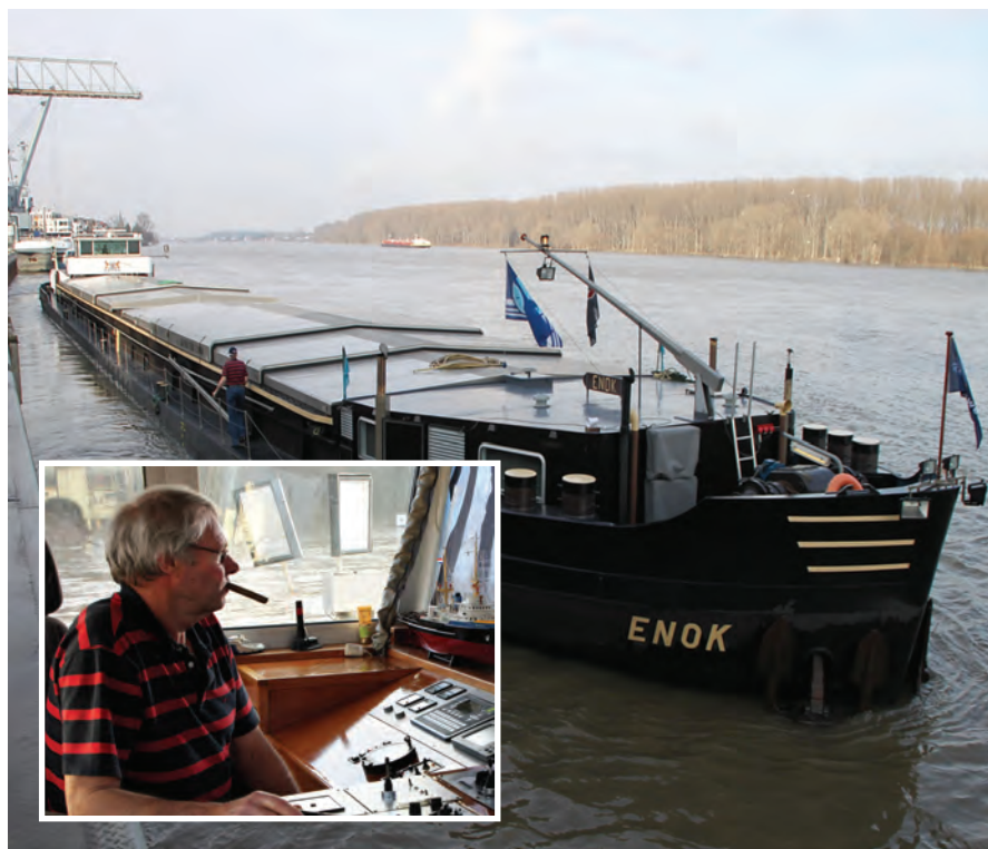
MV ENOK is worldwide the first motor vessel with a gearless, diesel-electrical Torque-Drive System. Inset: Rudi Koopmans (64) Captain of the vessel ENOK is absolutely satisfied with the new Torque Drive.
