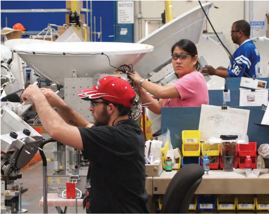
From closest to farthest: Nathen Gonderman, Production Assembler III; Felnor Lincer, Production Assembler III; Lamont Pollard, Production Assembler II. Sea Tel's Concord, Calif. facility is a lean factory, designed to get antennas out the door quickly. All manufacturing and testing stations are on wheels, allowing the entire layout of the factory floor to be reconfigured for any type of order.
