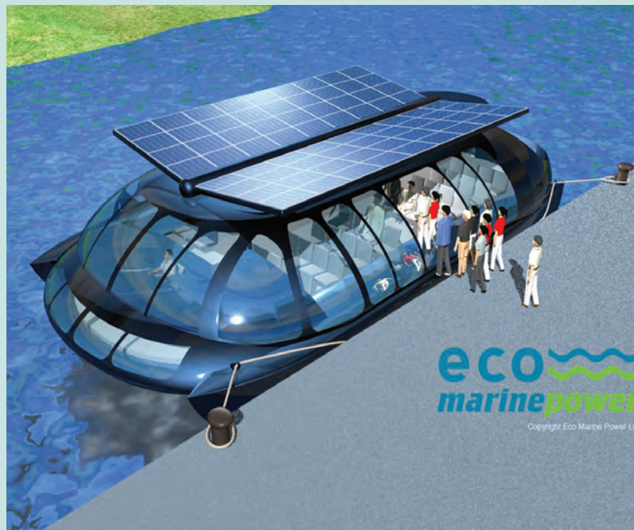
Impression of the eco solar ferry concept Medaka. The solar panels mounted on the roof are used to recharge batteries to help reduce fuel consumption and noxious gas emissions.
