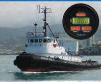
"I have used FloScan for over 15 years to identify our most fuel efficient towing speed. We monitor our GPS speed once we get strung out on the towline and then start backing off the throttles until we see a 20% drop
