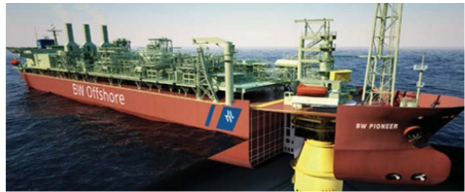
Below: BW Pioneer cut-out showing STP turret.
