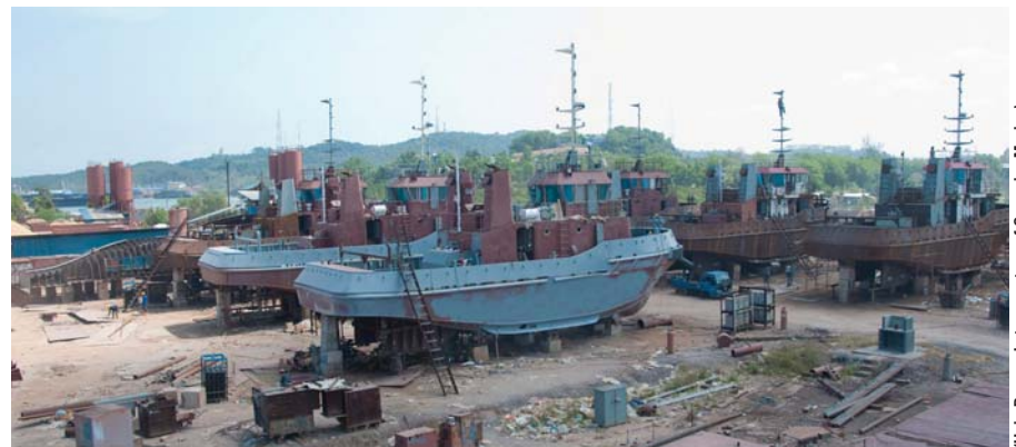
Eight 23.5-m tugs under construction at the Nongsa Jaya shipyard.
