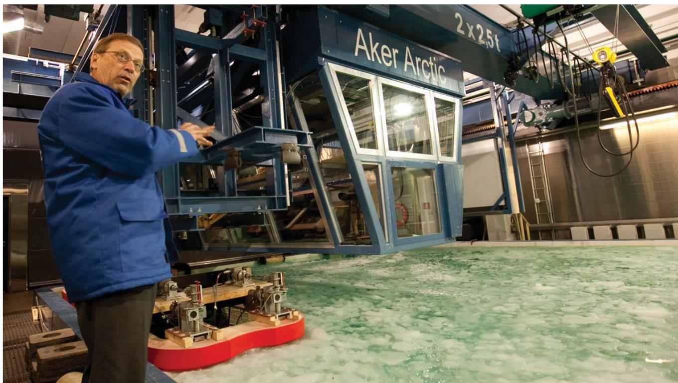
**Left & Right:** Aker Arctic Technology operates an ice model test basin 75m (229ft) long and 8m (24.4ft) wide, where all existing ice conditions can be simulated. Model tests are a cost efficient method to design ships and structures for Arctic conditions. Mikko Niini, Managing Director, provides insights to the facilities capabilities.
