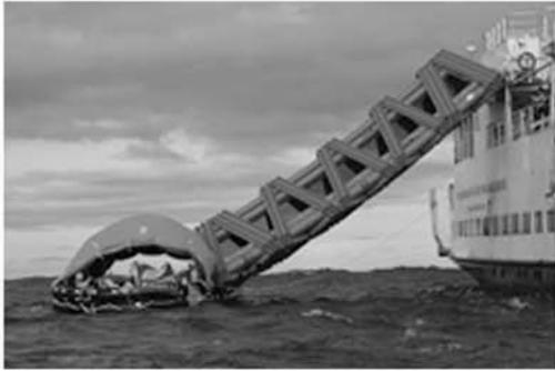
Zodiac's new MES MIS (Marine Evacuation System – Medium Inflatable Slide) is a double track slide SOLAS approved to evacuate up to 731 passengers in 30 minutes when used with Zodiac's Throw Over 150 person canopy life rafts. Also available with 100 person liferafts, 100 and 150 person IBA's. The new evacuation system is deployed at right angles to the ship's side and is available in four sizes covering freeboard installations from 4.7 to 9.3 metres.
