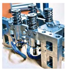
The VCM system varies valve timing and lift by interposing a high pressure oil chamber into the engine valve train.
