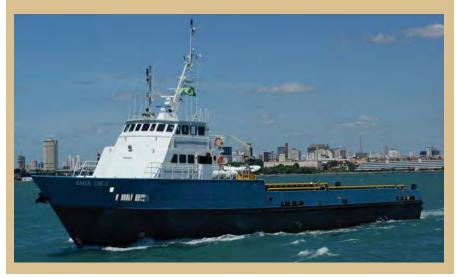
rate in a reverse osmosis water-maker. The craft has a maximum displacement of 100 tons when fully loaded. Powered by twin Caterpillar 3142E engines rated 634 kW (850 bhp) at 2300 rpm coupled to twin UltraJet 575 waterjets via ZF550 1.743:1 gearboxes, the craft has a top speed of 14 knots and a cruising speed of 11 knots. The Sistac Esperança was delivered to Sistac in August 2010, starting a new fleet of offshore vessels that will be in service in the Brazilian Campos Basin.
