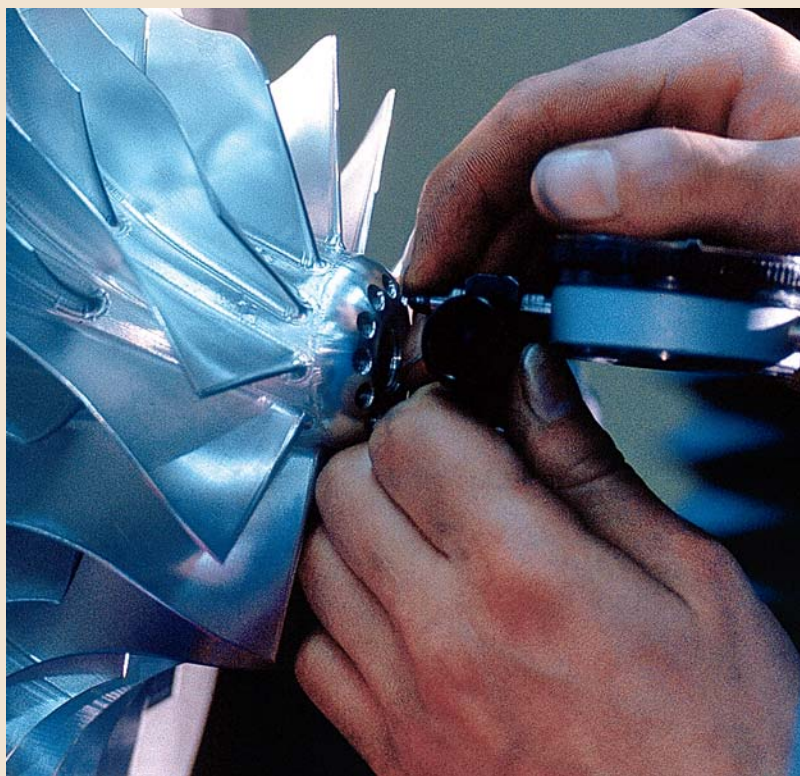
Above: Close attention to compressor and turbine geometry is essential to restoring turbocharger performance during overhauls. To ensure this, CPEX reconditioned parts are refurbished according to the same specifications as original parts.
