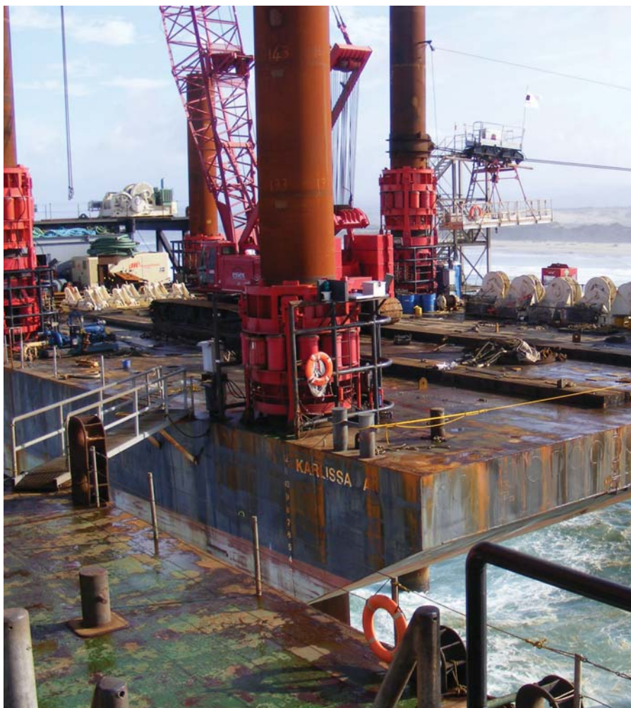
The jack-up barge Karlissa A, positioned at sea for wreck recovery
