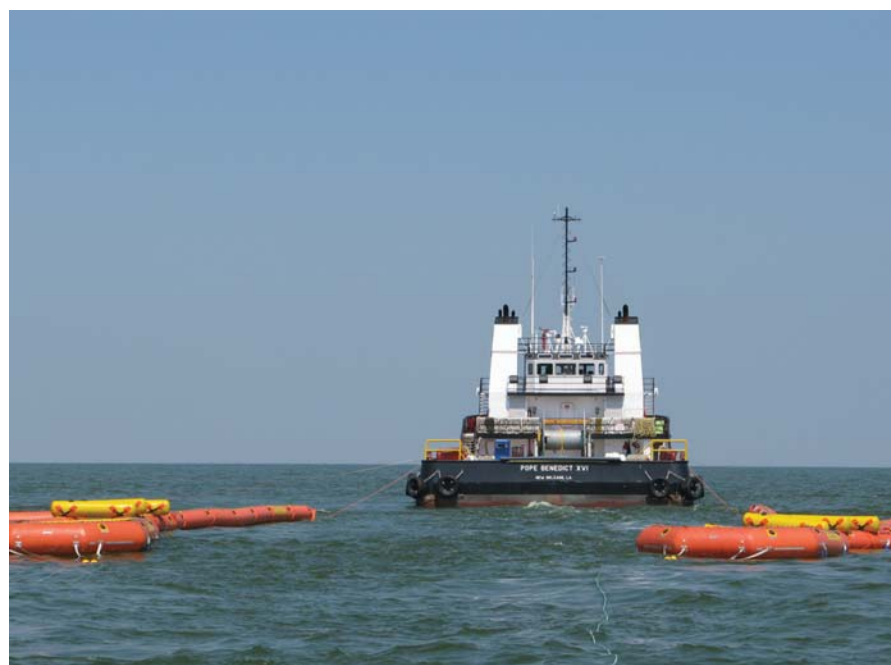
A Current Buster is towed behind the Pope Benedict XVI in skimming operations. The OSV, owned by Abdon Callais Offshore LLC, is under contract with BP for recovery operations.
