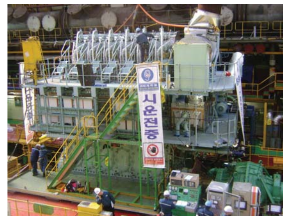
The first Tier II compliant MAN B&W engine, a low-speed two-stroke engine of 6S50ME-C7 type, built by licensee Hyundai Heavy Industries Engine & Machinery Division, was this spring installed in a Teekay shuttle tanker, to be delivered by Samsung Heavy Industries in July this year."
