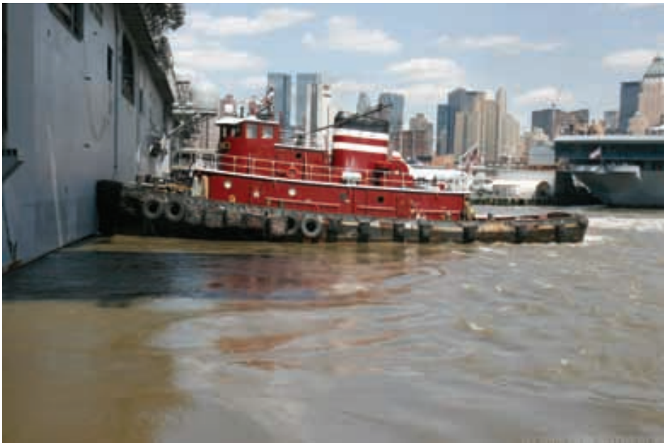
The single-screw J.P. McAllister, up from Balto, is one of four tugs keeping the Kearsarge against its dock. Nearby observers were surprised by the force they exerted. (Photo: Don Sutherland.)
