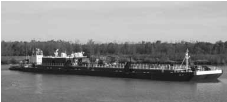
DBL 28 the 1st in a series of eight OPA'90 compliant, Lakes, Bays & Sounds, ABS and USCG certified tank barges delivered from Bollinger to K-Sea Transportation for use in harbor service in ports on the Northeast U. S. Coast.
