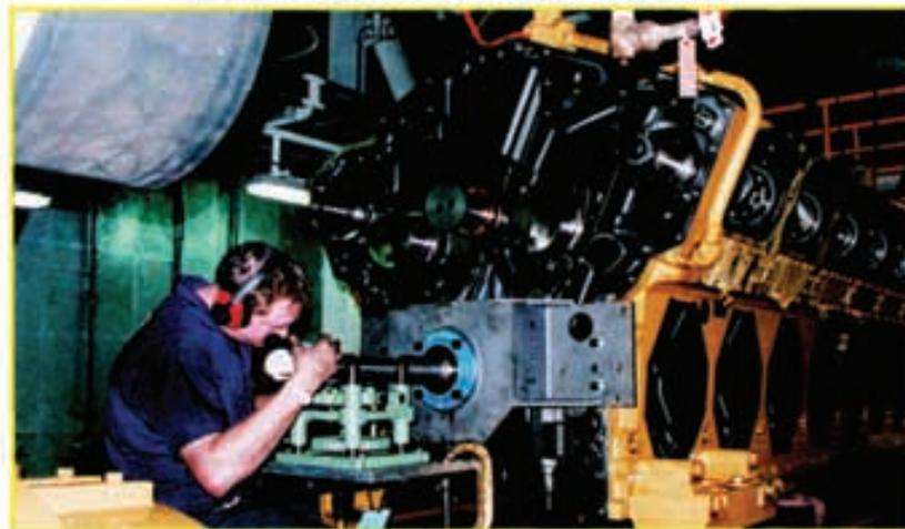
• CRANKPIN AND MAIN JOURNAL REFURBISHING While crankshaft is in engine
