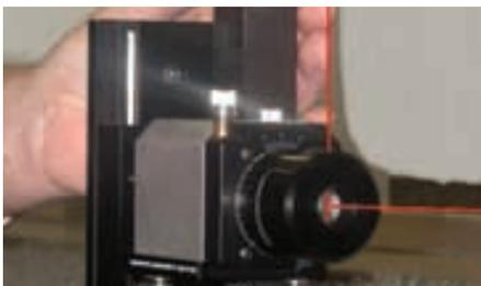
squareness and parallelism of machinery. These products allow plant personnel to check and align their own manufacturing equipment when they need to. The Right Angle Kit is ideal for checking machine beds, vertical cutting machinery, roll parallelism, squaring
