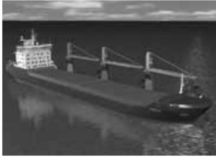
The first RTflex-50 two-stroke engine installed in China is a six-cylinder 9,720 kW engine for Rederi AB Donsötank's 19,500 dwt geared bulk carrier MS Credo. Built at Shanghai Edward Shipbuilding Company, the technically interesting vessel has a directly coupled Lips CPP propeller, a 2,000 kW shaft alternator, but no frequency cyclo converter. It is built to Finnish-Swedish ice class 1A Super.
