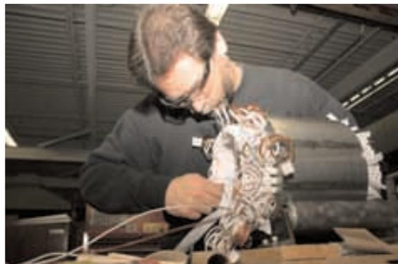
A technician inserts coils into the stator of an AC motor.
