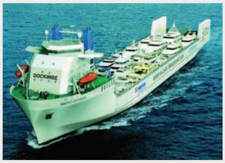
The new yacht carrier will be equipped with a 19,680 kW diesel-electric plant for propulsion, ancillary electrical power, and all shipboard electrical
