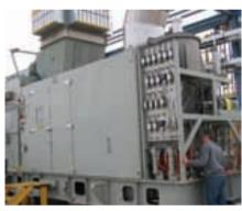
GE Transportation's marine gas turbine business delivered its LM500 aeroderivative Auxiliary Turbine-Generator Set (ATGS) for installation at the U.S. Navy's DD(X) next-generation destroyer land-based test facility in Philadelphia. This marks the first use of GE's LM500 genset for an electric drive application.
