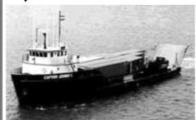
176' SUPPLY VESSEL 20' x 26' 100-TON CAPACITY STERN RAMP DUAL CATERPILLAR D399 DIESEL ENGINES DRY DOCK COMPLETED - MARCH 2005
