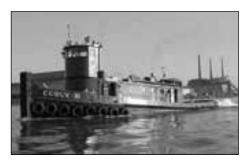
84' Model Bow - Twin Screw Flanking Rudders, Elevating Pilot House Tow Winch - Located in Michigan
