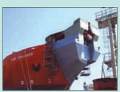
Following 40 days of rebuilding at Remontova yard in Gdansk, Poland, the Siri Knutsen was converted into a shuttle tanker. The company's KVOC tank system concept installed during the rebuilding.
