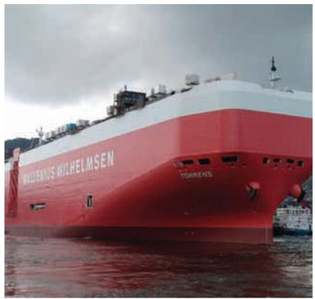
ity vehicles (SUVs). Emphasizing the 'high and heavy' freight carrying attributes of the design, the main deck has a maximum clearance of 5.20-m and has been strengthened for unit weights up to around 200-t, carried on special rolltrailers, and for a 60-t FLT (frontlift truck)
