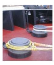
Schoellhorn-Albrecht Machine Co. has developed a new line of roller fairleads using state-of-the-art composite rollers to protect soft, synthetic rope from wear caused by traditional steel rollers. The composite matericombines al high strength, low water absorption and the
