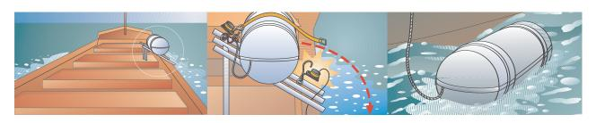
The Hammar remote release systems are designed to release heavy loads, such as liferafts or other objects, with little effort on all kinds of vessels. Two remote release systems are available:
