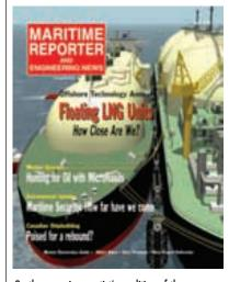
On the cover is an artist's rendition of the proposed Cabrillo Port — a floating LNG offshore vessel measuring 938 x 213 ft. (286 x 65 m) to be located approximately 21 miles offshore of California from the City of Port Hueneme. Cabrillo Port will house three spherical storage tanks into which the LNG is pumped from delivering carriers. See related article on page 34
