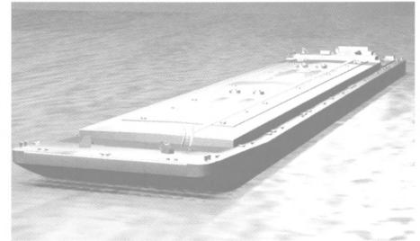
Artist drawing of the raked design 297.5-ft., 30,0000-barrel (BBL), double hull, hot asphalt tank barges Bollinger is building for Horizon.
