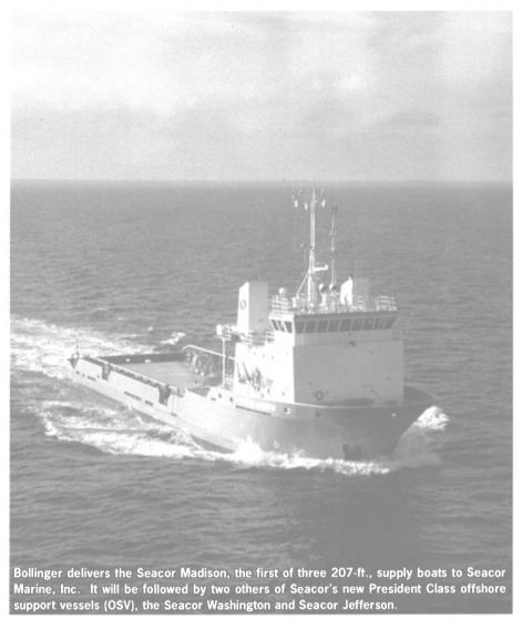
Bollinger Shipyards Lockport. La., has delivered the Seacor Madison, the first of three 207-ft., 4,750 bhp supply boats to Seacor Marine, Inc., Houston, Tex. It will be followed by two others of Seacor's new President Class offshore support vessels (OSV), Seacor Washington and Seacor Jefferson.
