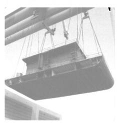
Just two weeks after delivering Carnival Cruise Lines' new 110,000-ton Carnival Glory, Fincantieri laid the first in a series of approximately 50 building blocks for a sister ship, Carnival Valor on July 10, 2003. The new 952-ft. (290.1-m), 2,974-passenger Carnival Valor, which is being constructed at Fincantieri's Monfalcone shipyard, is expected to enter service in December 2004.
