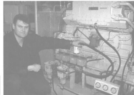
Cummins engine representative, Lutz Pauleburg , with one of the Cummins N14 engines that power the HADAG ferries.
