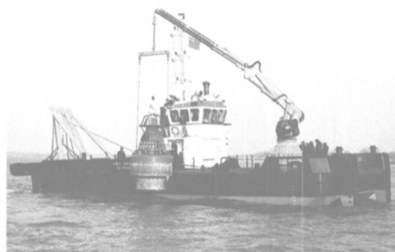
Damen Multi Cat 2510 Twin Screw Multi Purpose assistance and work vessel with propeller nozzles
