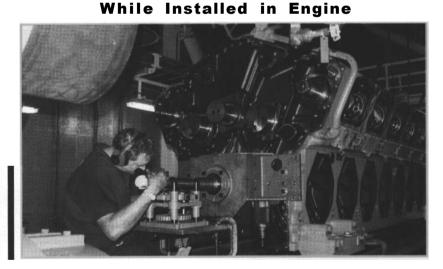
**CRANKPIN AND MAIN** JOURNAL REFURBISHING While crankshaft is in engine
