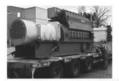
genset consists of Mak 8 M 20 with an output of 1,360 kW at 900 rpm for the container newbuilding 022 type WARNOW CV 2500. Since the acquisition by Kvaerner in October 1992, KWW has completed 35 container vessels, 32 of which of were equipped with Mak diesel gensets of the engine series M 20 and M 25.
