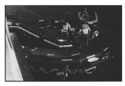
**Evacuation Slide System.** Designed specifically for Low Freeboard Vessels, it is a combination slide and platform. It provides speedy evacuation for all passengers - young, old and physically challenged. US Coast Guard Approved.
