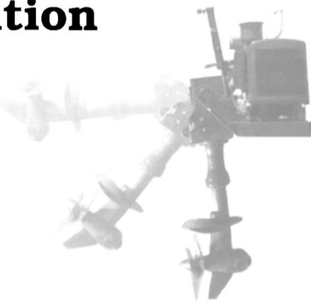
**Outboard and through-the-hull azimuthing drives**
