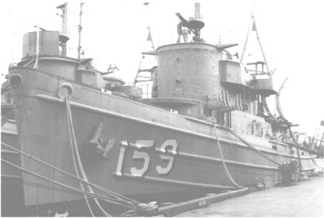
**TUG BALLISTICS** - **DISPLACEMENT:** 1,235 tons standard; **LENGTH:** 195 feet waterline, 205 feet overall; **BEAM:** 38-1/2 feet; **DRAFT:** 15-1/2 feet; **PROPULSION:** diesel-electric (4 Caterpillar D399 diesel engines); 3000 shp; 1 shaft; **SPEED:** 16.5 knots; **RANGE:** 15,000 n. miles at 8 knots, 6,500 n. miles at 15 knots.
