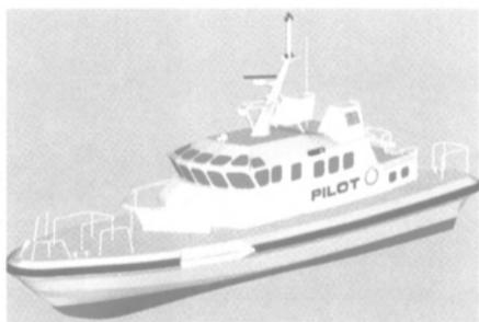
Kvichak Marine Industries has been granted the contract to build a 72 ft. (22 m) all-aluminum pilot boat for the Columbia River Bar Pilots Association of Astoria, Ore. Named Chinook, the vessel was designed by Camarc, Ltd. It is scheduled for an August 2000 delivery. Chinook is designed to survive a 360-degree rollover while maintaining a safe return to its mooring with crew and equipment intact.
