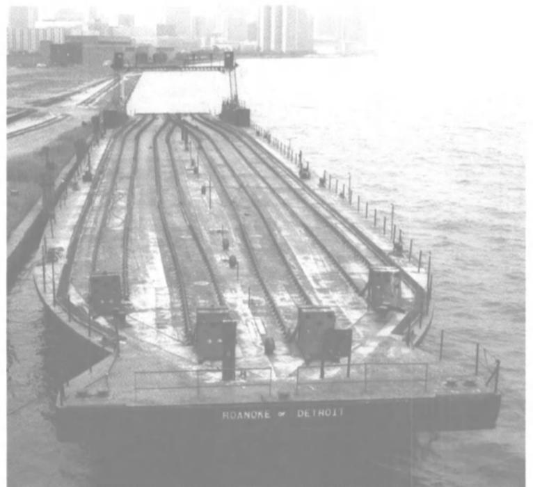
**ROANOKE, US 229316:** 369' x 57.3' x 20.3' Steel. 3327 GT; **BUILT:** Manitowoc, Manitowoc Shipbuilding Co. as Car Ferry, City of Flint 32; **CAPACITY:** Four tracks, 26 cars. **\$400,000** each OBO
