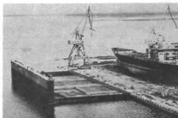
1. The Austral Envoy prior to launching on the shipyard's various modules of the ship were joined together to form it
