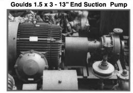
Model:3196 Material: 316SS Impeller: 12.75" CCW Reliance Motor HP:125 RPM:3570 Volt:440
