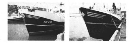
(Left above) 'Sunnanland' – virtually free of corrosion after <u>2 years</u> in service working in ice. The hull is protected with 2 coats of Jotamastic 87 and Seavictor Antifouling. The only maintenance required was fresh water cleaning, blastcleaning slipway support marks and application of 1 gallon of Jotamastic 87! Compare this with the photo (right) of 'Sunnanland's' sister ship, protected by conventional paints with obvious damage after only <u>1 year</u> in service.
