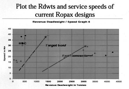
In examining the speed and capacity characteristics of the existing ferry fleet, Stuart Ballantyne found a "target void" which he seeks to fill with his innovative RoPax design.
