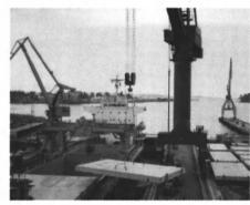
Astilleros Astander, which has built a solid reputation of providing quality service in a timely manner, significantly upgraded its facilities last year with the purchase and commissioning of a 200-ton tower crane, purchased from the ex Boelwerf yard in Temse. The 200-ton crane has considerably reinforced the lifting capacity of the yard's biggest drydock, drydock No. 2 which measures 230 x 33 m.
