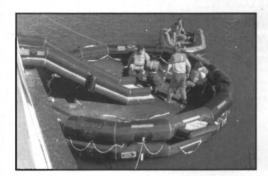
**Evacuation Slide System.**Designed specifically for Low Freeboard Ves-
