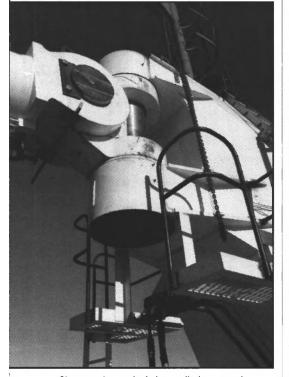
Closeup shows dual-pivot cylinder mounting, which allows the boom to swing and elevate easily. Duralon bearings support the vertical pin.
