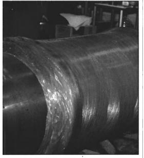
Duralon bearing is shown during manufacture, after fiilament-winding operation that combines fiberglass epoxy resin matrix with a woven Teflon and polyester fiber bearing element.
