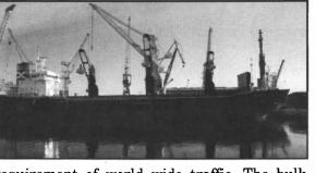
requirement of world wide traffic. The bulk carrier is classified in the highest Finnish ice class (1 A Super). It can visit the most northern Finnish ports, even under severe ice conditions, ensuring the energy management and raw material exports and imports.
