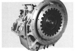
• More Power: ZF Marine Transmissions are rated for diesel engines from approximately 5 bhp up to 10,000 bhp — with ratios to meet your needs, from 1.0 to 7.6:1.
