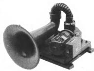
Model S-120 Piston Horn Chosen for use on aircraft carriers as well as commercial vessels over 200 meters in length, the S-120 utilizes an oscillaling piston driven by 7-1/2 horsepower 3 phase 220/440 volt electric motor producing 143 dB and a fundamental frequency of 94 Hz in 1/3 octave band at one meter.
