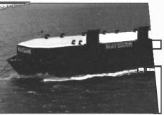
Conrad Shipyard, in Morgan City, La., has delivered a new RoRo freight warehouse barge to Maybank Shipping Company, Inc. Classed ABS Maltese Cross, A1, All Oceans and USCG certificated, the barge is 278 ft. long, 80 ft. wide and 18 ft. deep, and features a shaped bow for improved towing in all weather conditions.
