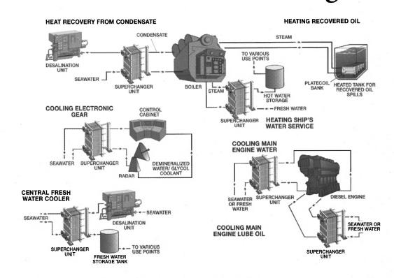
Naval ships, fleet oilers, commercial containerships, tankers and dredges are successfully finding new ways to operate more efficiently at lower cost, by utilizing Tranter's unsurpassed plate-type heat exchanger technology. Schematics presented hears illustrate upricel ways they are doing it.
