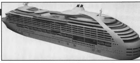
Kvaerner has the knack of making fantasy a reality. Here is the concept of an "ultra-sized" cruise ship for Royal Caribbean Cruise Lines. The first of three of the 136,000 grt, \$500-million vessels is under construction at Kvaerner Masa-Yards now.
