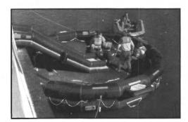
**Evacuation Slide System.** Designed specifically for Low Freeboard Vessels, it is a combination slide and platform. It provides speedy evacuation for all passengers - young, old and physically challenged. US Coast Guard Approved.
