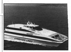
Westamaran 4200 Mirage was delivered to the owners Strintzis Lines, based in Pireaus, Greece, to sail in Greek waters. This is the first Westamaran built Batservice Holding A/S, and is the largest catamaran built at the yard. The 137.8 ft. (42 m) vessel has a 386 passenger capacity. The main engines are two MTU 16V 396 TE74L at 2,000 kW and two MTU 12V396 TE74L at 1,500 kW. The vessel is also equipped with a motion dampening system from Maritime Dynamics Inc., including T-foils and flaps.
