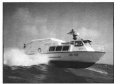
Patrol Boat to the U.S. Army Kawajalein Atoll, in Marshall Islands. With a 15 ft. (4.6 m) beam, and a 4.5 ft. (1.6 m) draft, the vessel is powered by a pair of 8V92TA Detroit Diesels. Maximum speed is 35 mph. Special equipment onboard includes crew cabin with galley and head; dive/rescue platform; 800-gal. fuel tank; 48,000 BRU air conditioning; emergency blue strobe light and 12 kW water cooled diesel generator.
