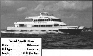
Beam: ............33 ft. (10.1 m) .....diesel engines .....ZF BW450D Gensets: ..............Cummins/ . . . . Onan MCGDA 70 kW Hydraulics System: . . Bird-Johnson Radar: . . . . . . (2) Furuno FR 8051 ..... (2) Furuno FM2610 .Furuno GP 80D DGPS Depth Sounder: .... Datamarine **DDM 600** Fuel Capacity: ..... .2,800 gal. .200 gal. Fresh Water Capacity: .. .300 gal. 33 knots Speed (light): . . . . . . . . . . . . . . . . . . 37 knots
