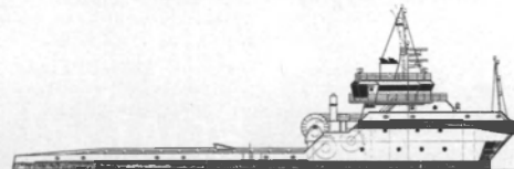
220'x48'x20' 8000 HP Anchor Handling Tug Supply Vessel
