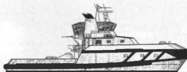
111'x39'x20' 6000 HP Anchor Handling Tug
