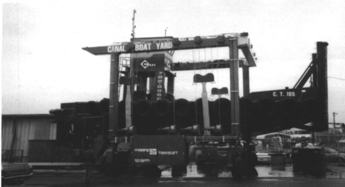
A Marine Travelift model 50BFM mobile boat hoist during a haul-out at Canal Boat Yard, Seattle.
