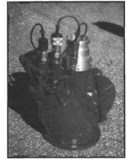
Ro-Clean Desmi's DOP-160 Submersible Screw Pump.
