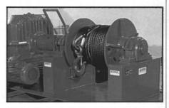
Jeamar's electric winch is designed to pull railcars in the former Soviet Union
