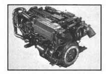
Yanmar has introduced a new lightweight, six-cylinder diesel engine into its line of marine products. The 4.2 L, 899 lb. vertical four-stroke, fuel-injected engine uses a four-valve intake-exhaust system and is freshwater cooled. The new 6LP-STE develops 300 hp at 3,800 rpm and measure 47.4 x 26.2 x 29-in.
