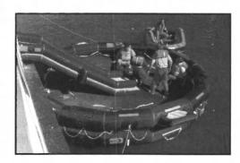
**Evacuation Slide System.** Designed specifically for Low Freeboard Vessels, it is a combination slide and platform. It provides speedy evacuation for all passengers - young, old and physically challenged. US Coast Guard Approved.
