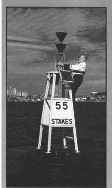
A Tidewater solar-powered steel buoy is shown being checked at its moorings outside Poole Harbor in southern England.
