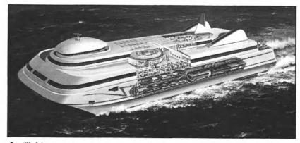
Seaflight: 110m, Passenger, Cars, Bus, Gas Turbine
