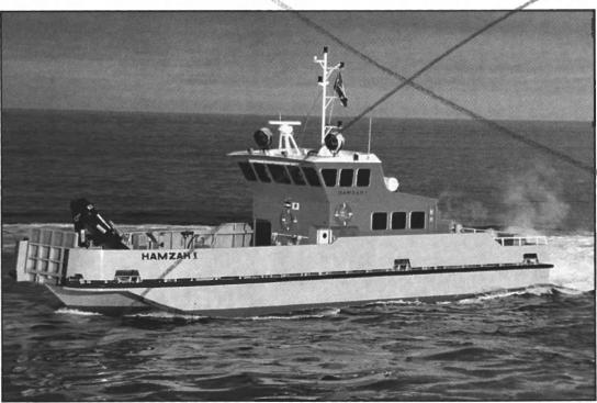
Hamzah 1 is a monohull oil combat vessel built by Amble Boat Co. The vessel was a gift from Japan to Jordon.
