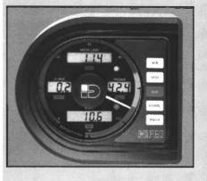
Datainstrument AS has introduced Mipeg 2000, an electronic load indicator and crane monitoring system designed to provide crane operators with the necessary information to meet world-wide government to irements for crane safety. The system comprises and, everturning and angle control with a micro computer that calculates the sensor data and provides an image of the crane's utilization on the operator's display.
