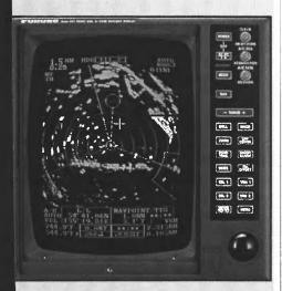
Furuno has replaced its FR7041 daylight viewing radar with an updated 12-in. X bank model the FR7061. The FR voice provides a 5t percent increase in output power, a maximum range scale of 64 nm, optimized userfriency software and True Echo Trail for accurate target tracking. Standard features on the FR7061 include dual EBLs and VRMs, EBL/VRM offset, off-center, zoom, echo trail, echo plot, and aural/visual guard zone alarm.
