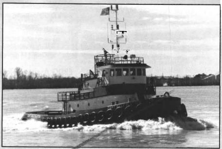
in tight spaces. This vessel is also outfitted with an stainless steel tow bits and bullnose, which will reportably help prevent chafing and wear of the Spectra 900 fiber rope slings. This is the third tug in the Bisso fleet to be outfitted with these slings.
