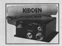
The Koden KBR-91 differential GPS beacon receiver is capable of pinpointing locations within 1 ft. by automatically locking onto the strongest differential bracon signal it and detect. The KBR-91 recognites Type 1 Type 2 and Type 9 broadcasts, and it is compatible with the RTCM-104 interface on most differential-ready receivers.
