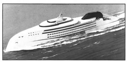
Trimaran HST-800: 40 Knot, Steel Trimaran, Gas Turbine, Passengers, Cars, Freight
