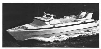
Monohull HSM-150: High Speed, Aluminum, Diesel, Passengers, Cars
