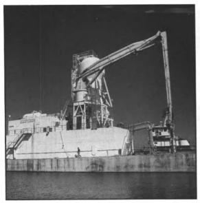
Intended Service: General discharge of bulk cement from ship to barge, injunct Lakes, Bays & River
